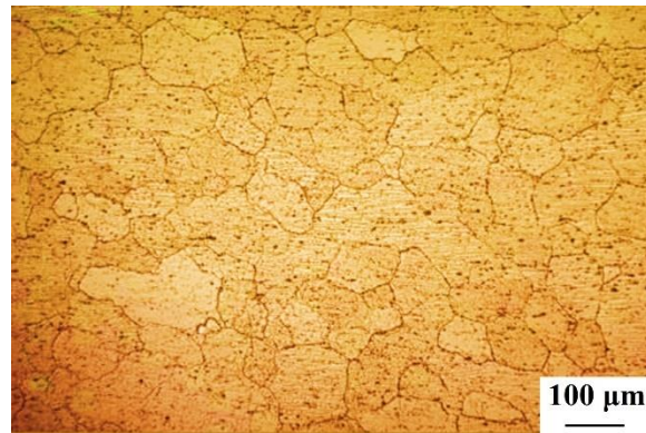
Figure 4: Microstructure of weld stir zone, (a) 1000 rpm, (b) 1200 rpm, (c) 1400 rpm, (d) 1600 rpm, (e) 1800 rpm
