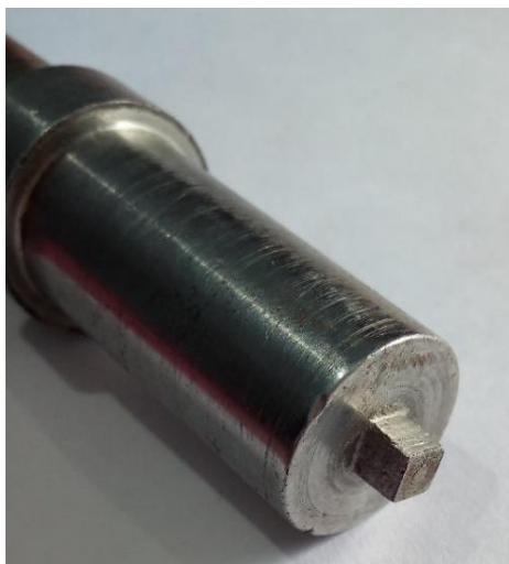
Figure 2: Cross section of friction stir welding tool
