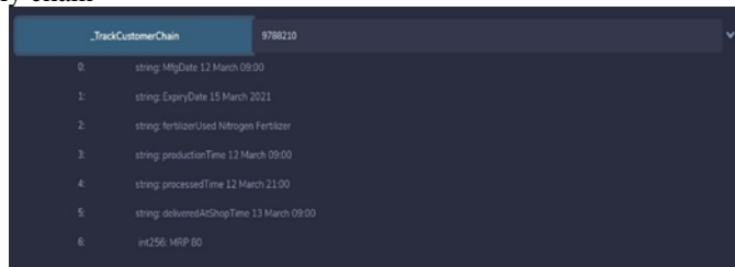
Once the vendor is done with the registration and the staking process, then the smart contract allows the vendor to update their corresponding supply chain data into the Blockchain. fig 6.5, Producer updating his/her Production data into the Blockchain.
