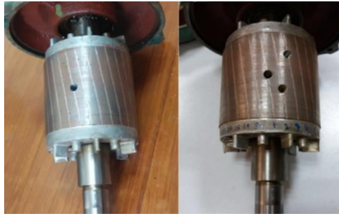
Fig. 4. Artificially Created Broken Rotor Bars
