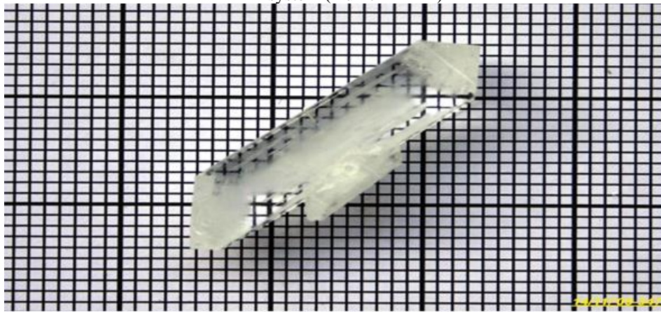
Fig. 2 A typical grown crystals of ADP taken out of the system (1 unit = 2 mm)
