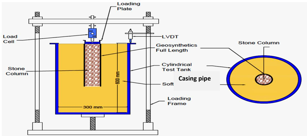
Figure 2: Schematic diagram for load test on single stone column in a unit cell
