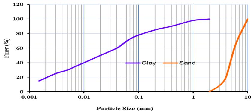
Figure 1: Grain size distribution of clay and stone aggregate for laboratory model test
