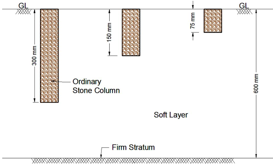
Figure 3: Laboratory model consideration for floating Stone column with different length consideration
