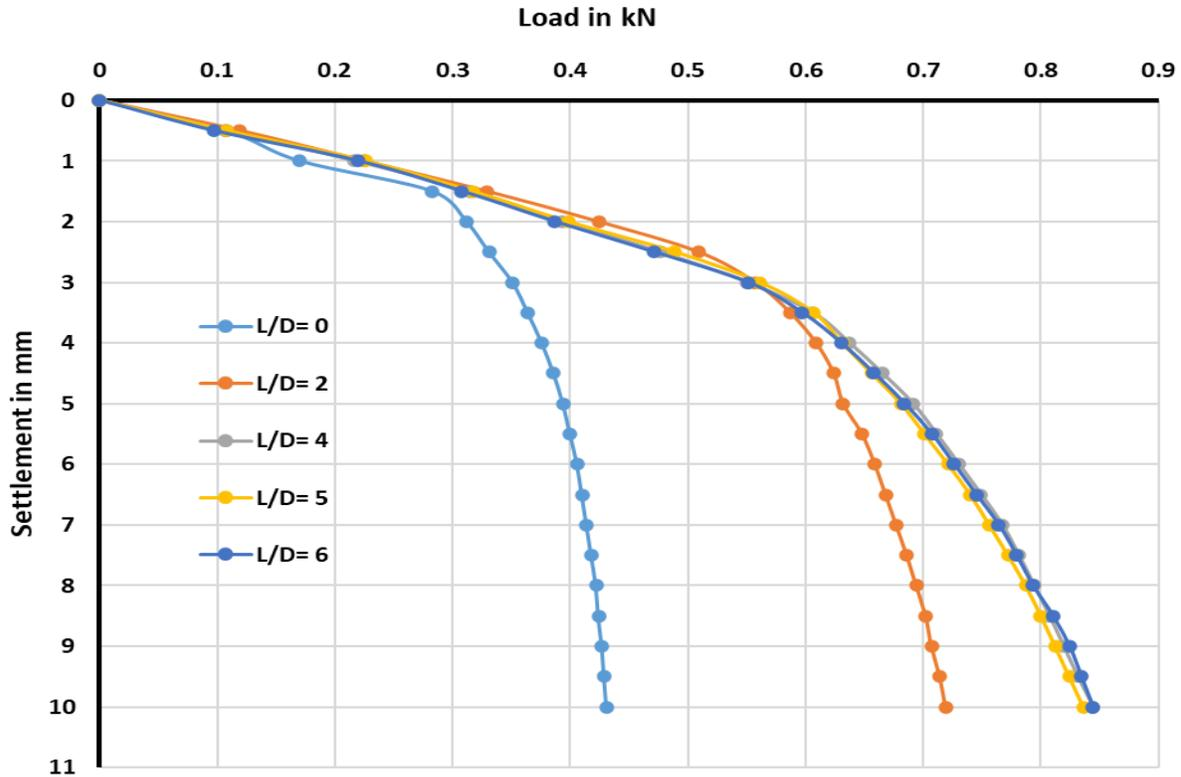
Figure 4: Load Vs Settlement for 60 mm Plate & Floating Stone Column at 10 mm prescribed settlement
