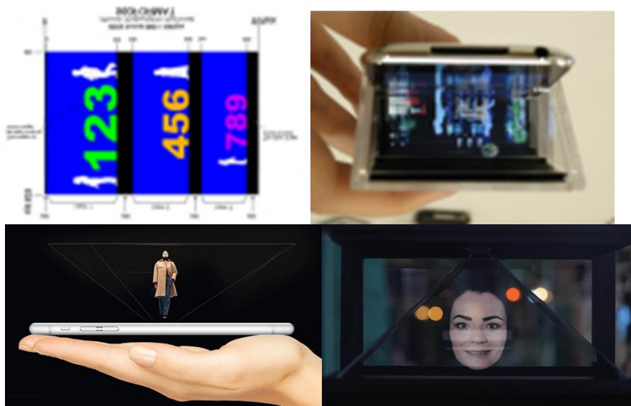
Figure5. A fashion show that embodies the 3D hologram principle using a polyhedral reflector with a mobile phone (The studio k)
