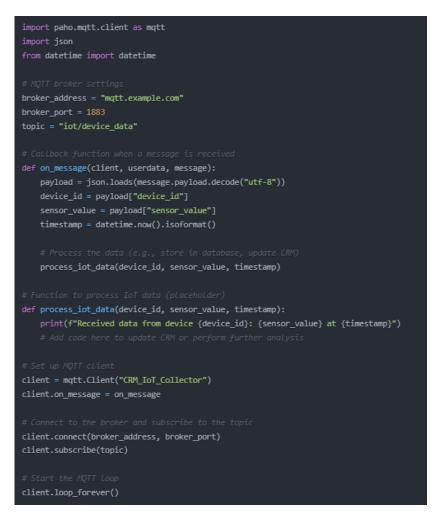
This script sets up an MQTT client that listens for IoT device data on a specific topic. When data is received, it's processed and could be integrated into a CRM system for further analysis and action.
