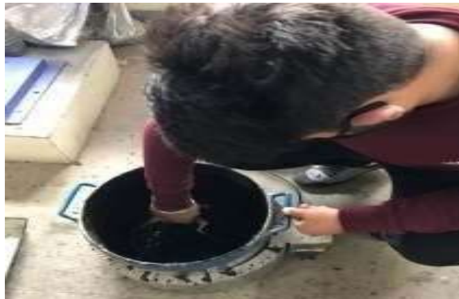
Mixing shredded plastic with aggregate
