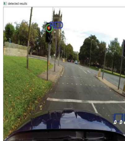
FIGURE 1: The Red Color Traffic Signal is Detected.
