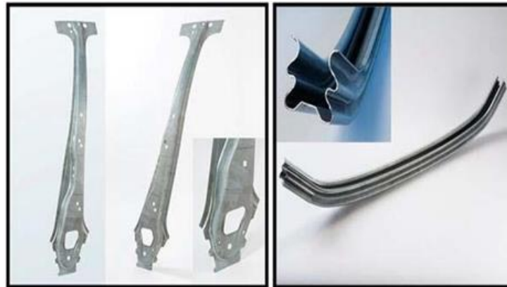
Figure 5. Typical application of TRIP steel for manufacturing B-Pillar reinforcement and Bumper cross member respectively (Reprinted from [76])
