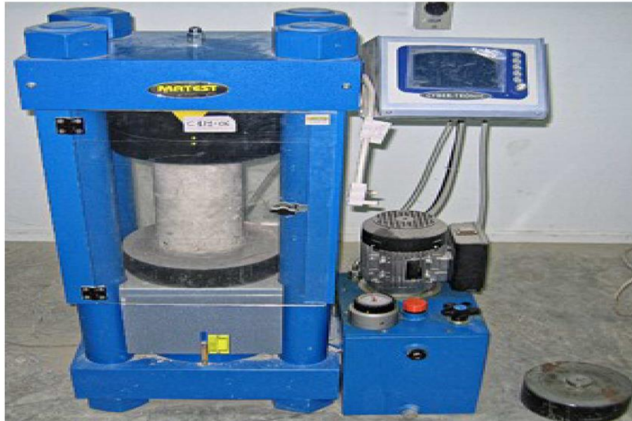
Figure 5: Compressive strength test process images
