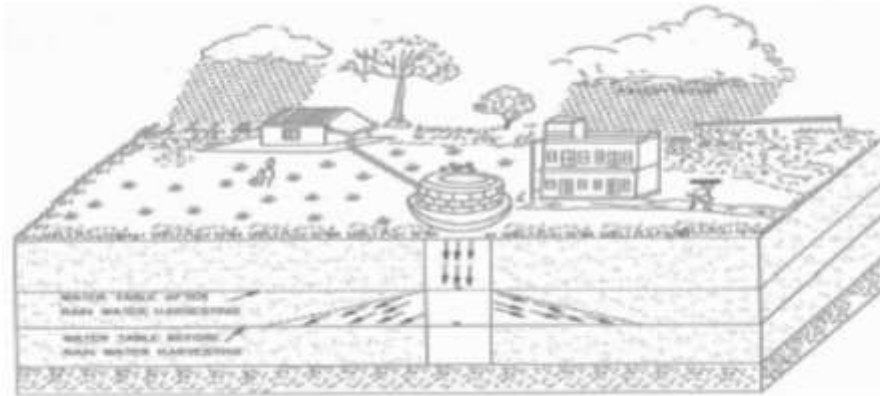
Figure 2.7 Recharge of dug wells and hand pumps
