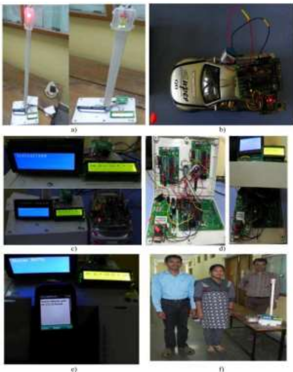
Fig. 5. Proposed model images transmitter and receiver. (a) Pole status at different condition. (b) Transmitter (ZigBee). (c) LCD display at receiver. (d) Detailed image
