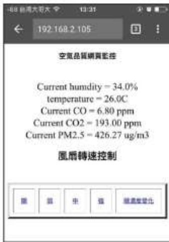
Fig. 6. The developed website for fan control.
