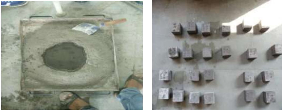
Fig. 1 Preparation and casting of masonry mortar and cubes
