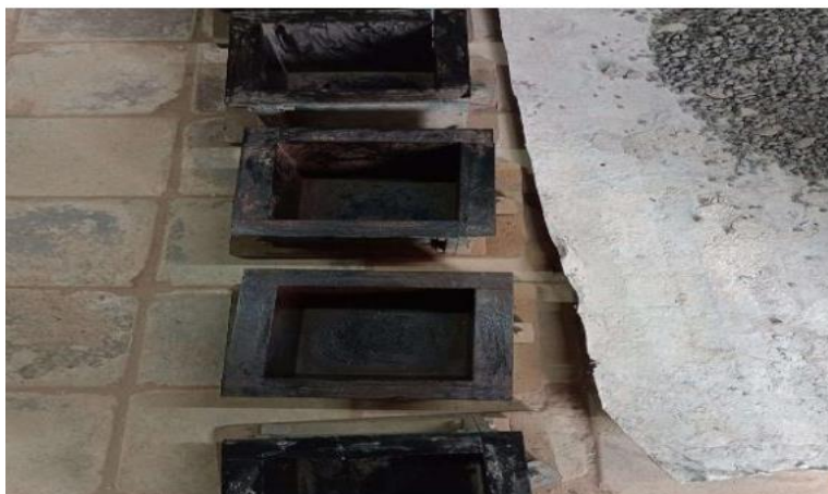
Fig 3.9 Oiling of Mould
