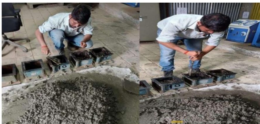
Fig 3.10 Casting of Cubes
