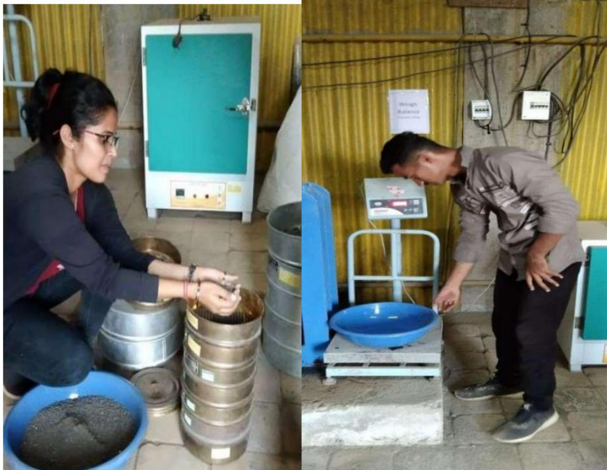
Fig 3.7 Fineness Modulus Test
