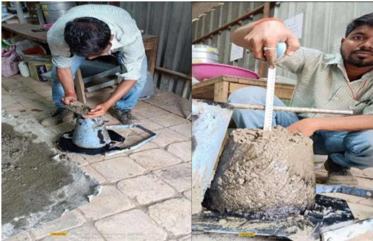
Fig 3.8 Slump Cone Test
