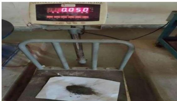
Fig 3.2 Passing Weight of Crushed Aggregate
