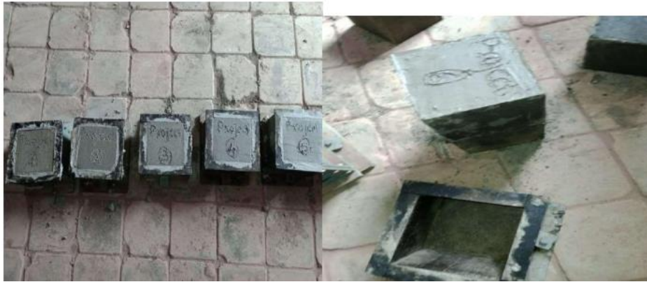
Fig 3.11 Removal of Cubes
