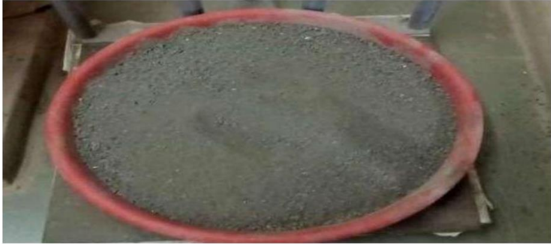
Fig 3.6 Fine Aggregates for Water absorption Test Percentage Water Absorption of Fine Aggregate Sample = 6.34%
