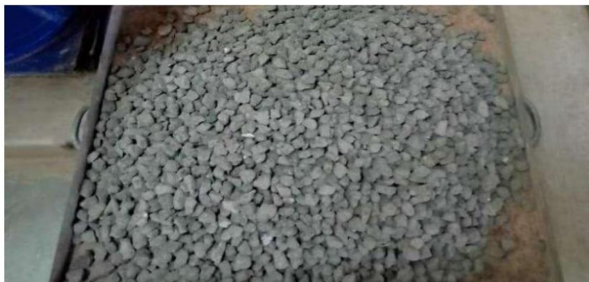
Fig 3.5 Coarse Aggregates for Water absorption Test
