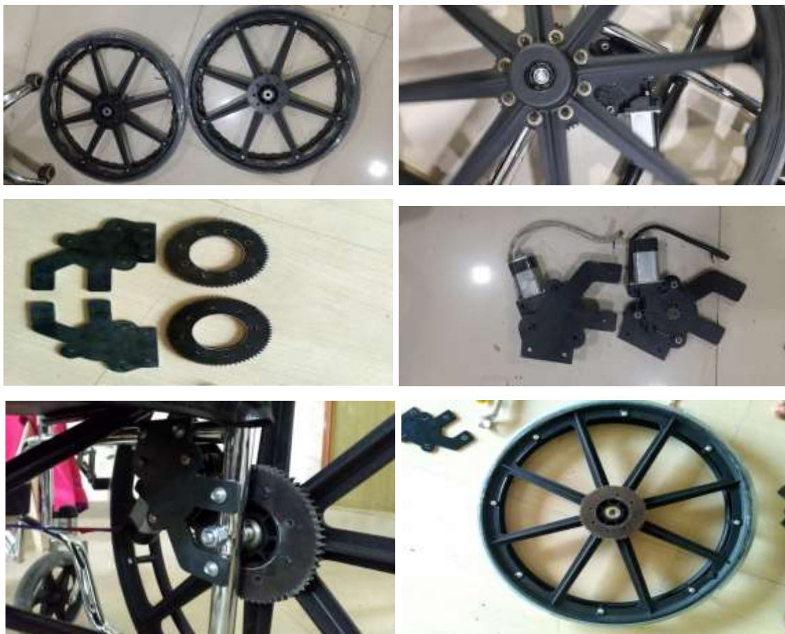
Figure 4: Wheels alignment and gear fixing.
