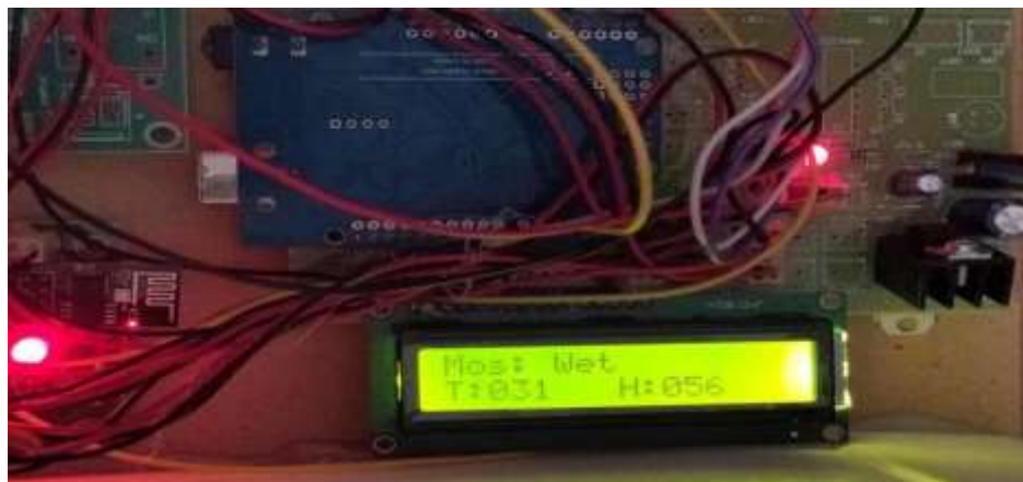
Figure 5 Lcd indicating the soil is wet
