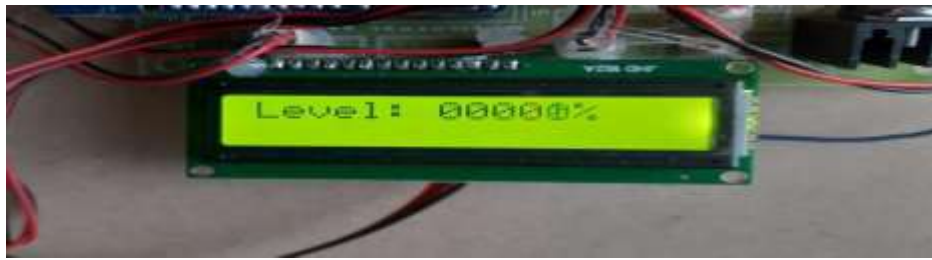
Figure 6 Lcd displaying the level of the bin.
