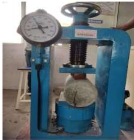
Fig. 7: Tensile strength test on cylinder.
