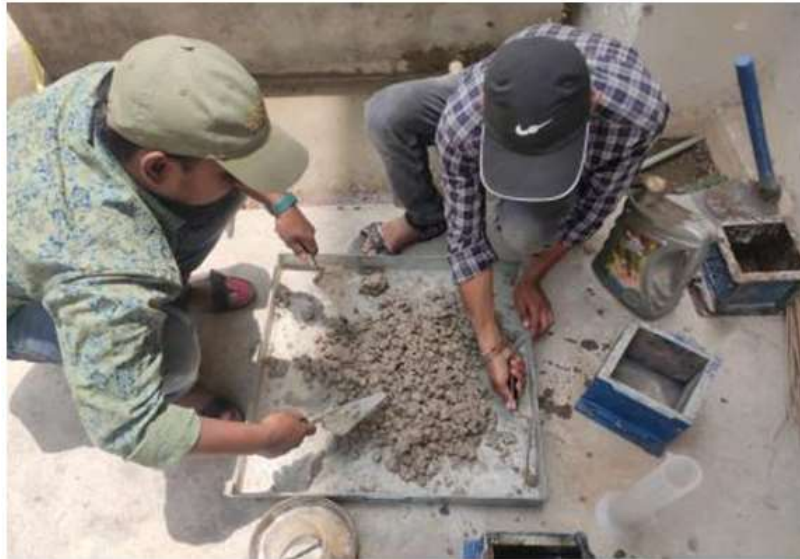
Fig. 10: Cube casting with AAC.
