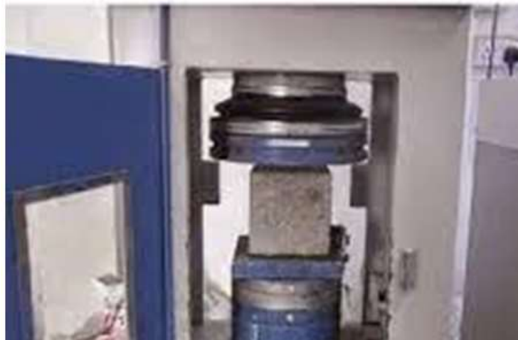
Fig. 13: Compressive strength testing of cubes.
