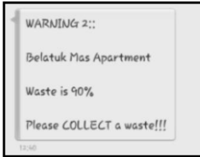
Fig. 7: SMS sent by the system when waste reaches the level of 90% full.
