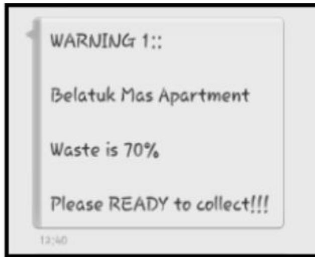
Fig. 5: SMS sent by the system when waste reaches the level of 70% full.
