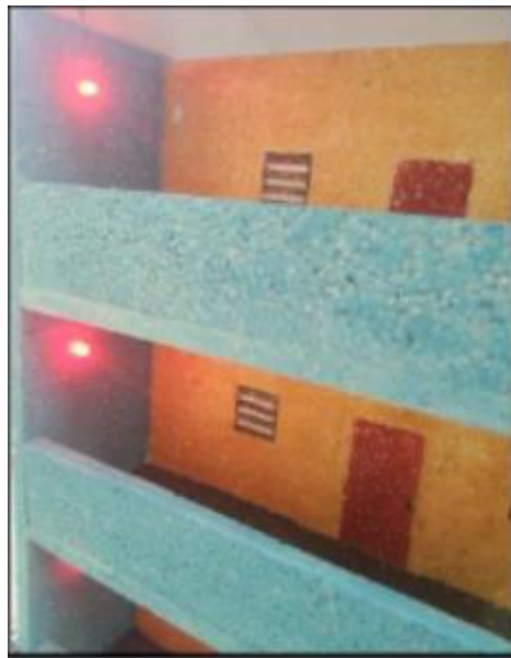
Fig. 6: Red LED is turned on when waste reaches the level of 70% full.
