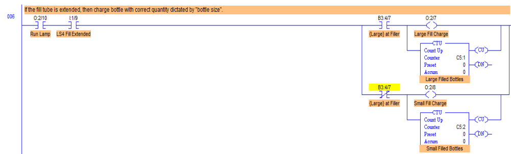
Figure.8 Fill the bottles according to their sizes
