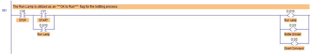
Figure.3 Initialization of “Run Lamp, Bottle Griner and Divert Conveyor” outputs
