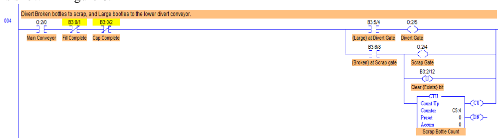
Figure.6 Divert broken bottles to scrap and large bottles to lower divert conveyor
