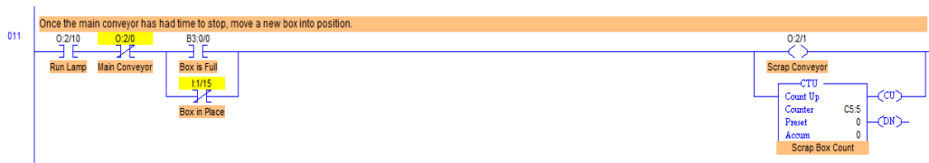
Figure.11 Activate scrap conveyor and scrap box counter
