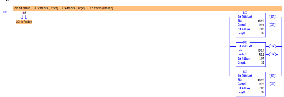
Figure.5 Tracking bottle exist, large bottles and broken bottles
