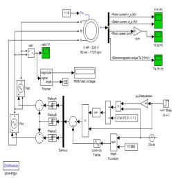
SIMULINK blocks. Its output goes through controlled voltage source blocks before being applied to the asynchronous machine block's stator windings. The machine's rotor is short circuited. Its stator leakage inductance is set to twice its actual value to simulate the effect of a smoothing reactor placed between the inverter and the machine.
