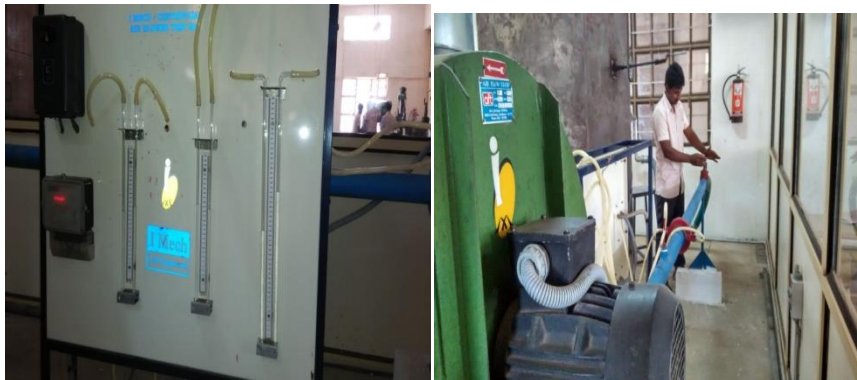
Fig-1 Centrifugal blower with manometer measurement set up
