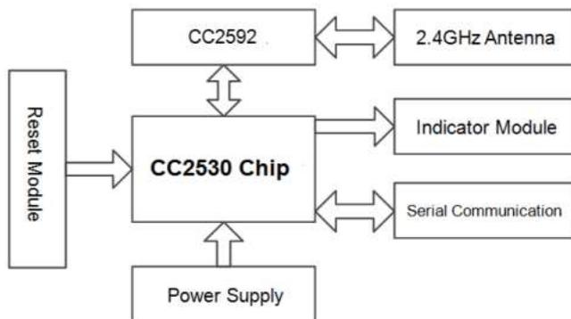
Figure 6. Ordinary routing device hardware structure
