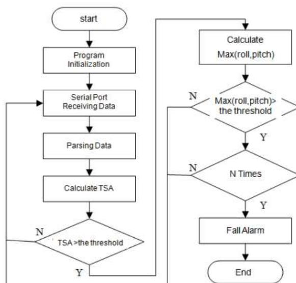
Figure 4. Fall detection process
