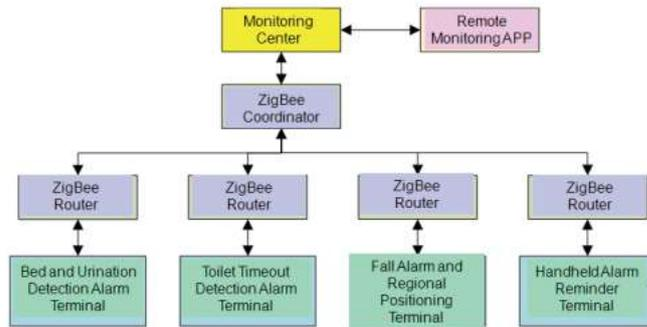
Figure 1. System architecture
