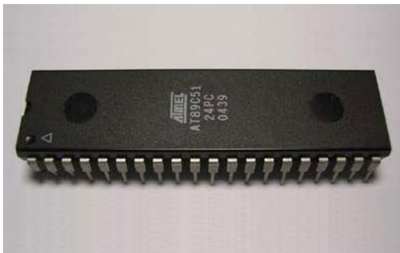
Fig. 3: AT89C51 microcontroller chip
