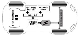
Figure 3Fuel Cell Electric Vehicle
