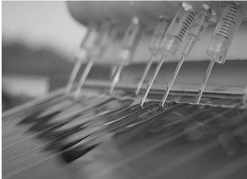
Fig. 16. A line of nozzles creates a water on PV module
