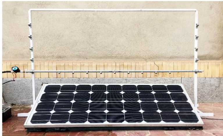
Fig. 12. With its unique experimental configuration, a photovoltaic module is cooled by water spray.
