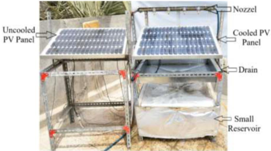
Fig. 6. Photovoltaic panels are being tested in this arrangement.
