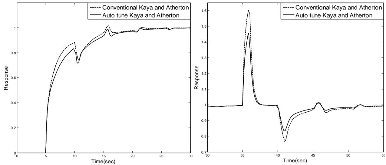
Fig. 5. Set point and load responses of the proposed auto-tuning modified Smith predictor and conventional Smith predictor with perturbed process model given by relation (15).
