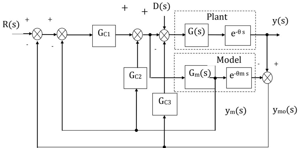
Fig.2. Modified Smith predictor structure [8].
