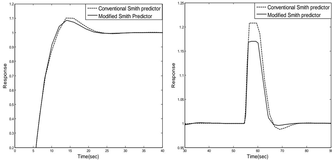
Fig. 1 Set point and load responses of the conventional [4] and modified Smith predictor [8] for delay dominated integrating process.
