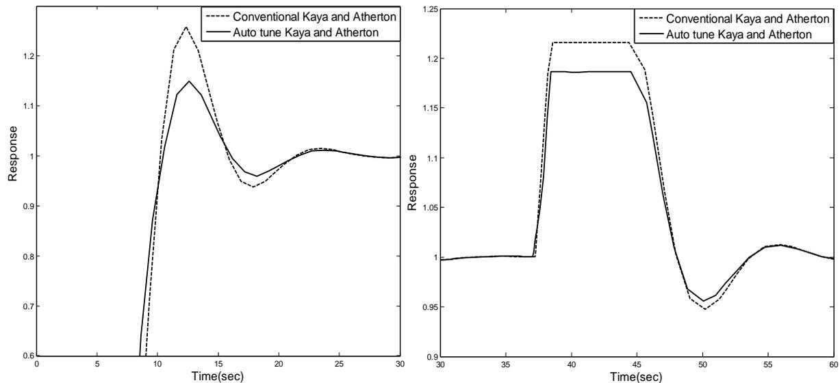
Fig. 6 Set point and load responses of the proposed auto-tuning modified Smith predictor and modified Smith predictor given by relation (16).
