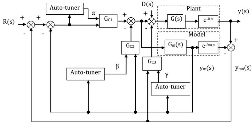
Fig. 3 Auto-tuning scheme with modified Smith predictor control technique
