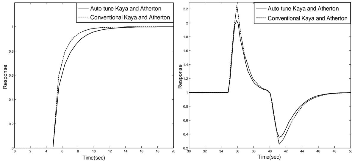
Fig. 4. Set point and load responses of the proposed auto-tuning modified Smith predictor and conventional Smith predictor are given by relation (14).
