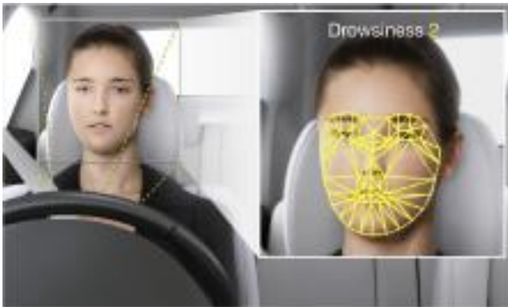
Fig. 7. Driving State Monitoring System in DENSO
