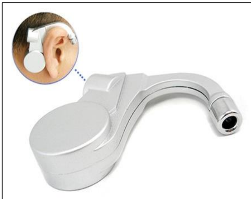
Fig.4.Inclination Detection Vibration Sensor
