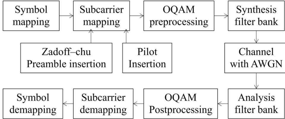
Fig. 1: Proposed block diagram for FBMC.
