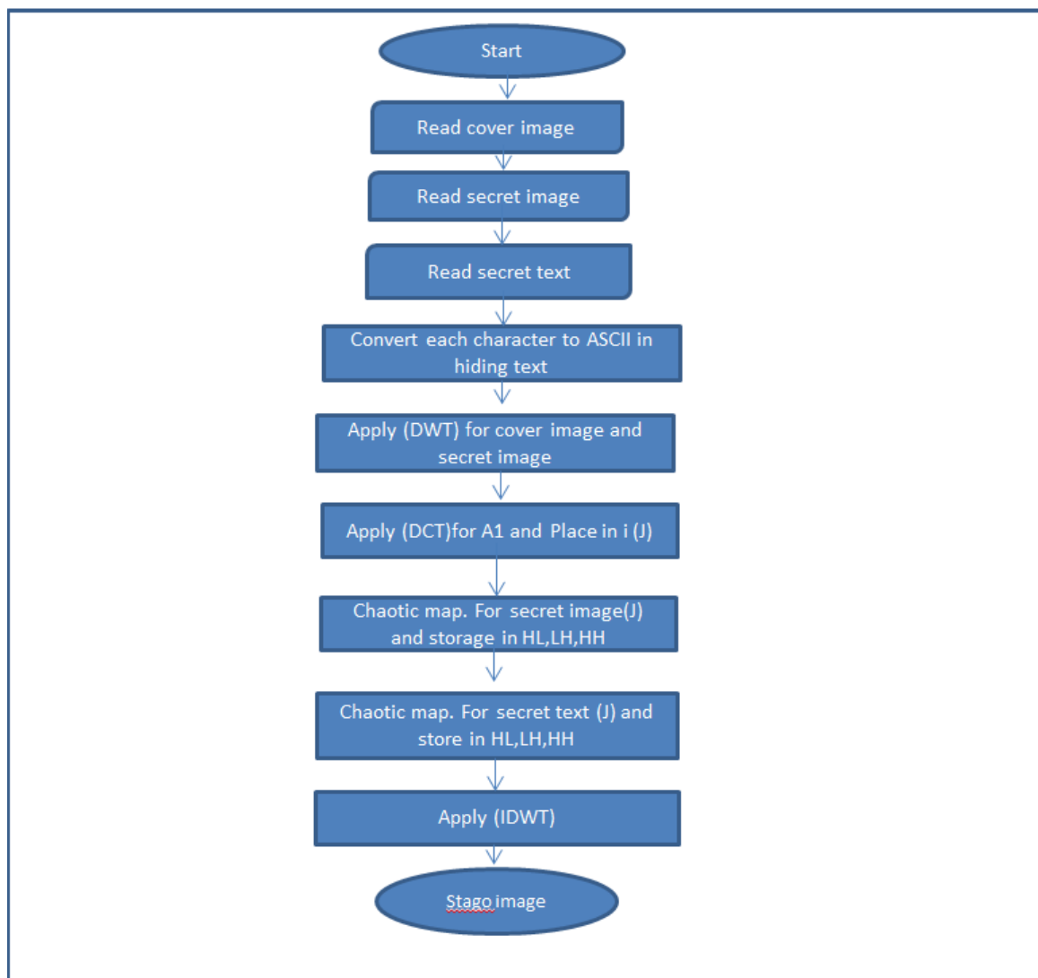
Figure (3.3) Depicting the embedding algorithm flow chart of hiding secret image and secret text
