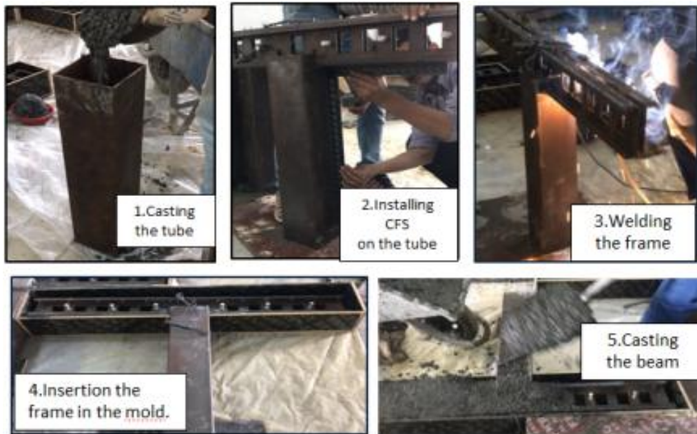
Figure 6. showing the casting of specimens
