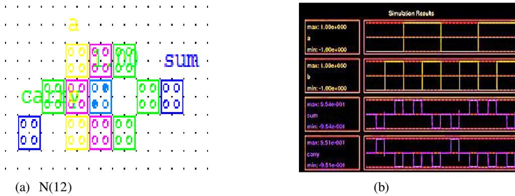
Figure5. Proposed QCA Half Adder (N12) (a) Layout (b) Simulation Waveform
