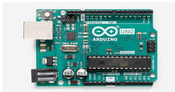
Figure.7. Arduino UNO board that is typical being used in projects.
