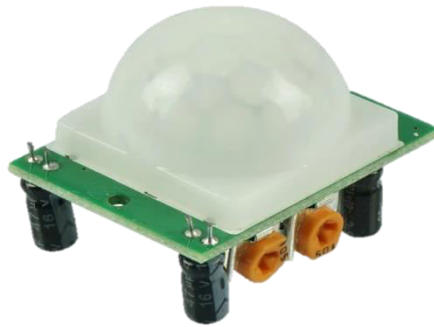
Figure.6. PIR motion sensor that is being used as an input in RomLIC design.
