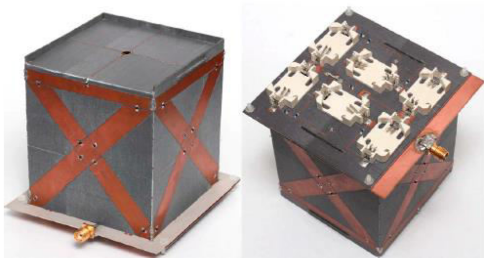
Figure 8. The fabricated prototype of pattern and polarization reconfigurable antenna
